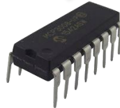
MCP-3008 8-channel 10-bit ADC
